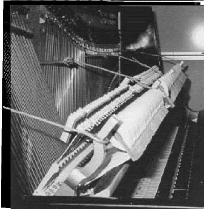
Photo 1 — (ABOVE) Action hanger wire shown securing action bracket to bolt. Photo 2 — (LEFT) End view of action tilted out for access, secured by four action hanger wires.
